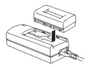
The CHARGE lamp lights red when charging starts. It turns off when the battery pack is fully charged. In the case of a fivebattery charger, when charging starts, the CHARGE lamp glows red. It then glows green when the battery packs are fully charged.
